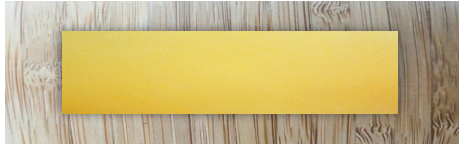
PU-50 film, dimension: 1 × 2 cm thickness: 500 μm
