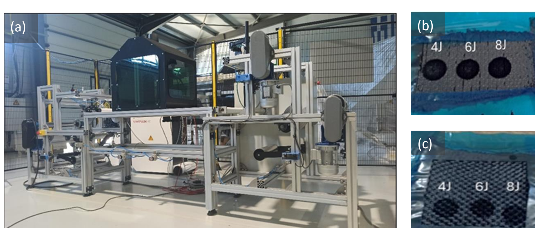
Fig. 3: (a) Image of the R2R pilot line (ADA), LrGO spots employing 4, 6 and 8 J on (b) PA and (c) PES textiles.
